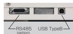
● A PC connector (USB Type B) is installed on the back of the unit RS485 (left side), USB TypeB (right side)
