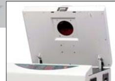
● the receiver of sensor is installed on the back of the lid.
